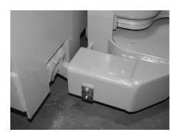
The linkage is reassembled, and reinforced, boxed in and tied into the chassis of the power head.
