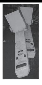
The forks and battery compartment of your pallet truck is completely apart. Reinforcement plates are added and the battery compartment along with the forks are widened to the correct width.
